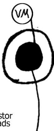
5. solder VM (red wire) to round copper tape pad on back side.
