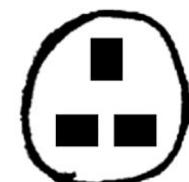
1. stick 3 copper tape pads on front side of kapton surface.
