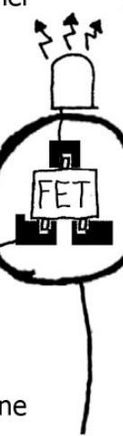
9. solder metal wire touch electrode to transistor gate (G) on front side.
