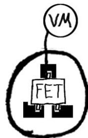
4. solder VM (blue wire) to the transistor drain (D).
