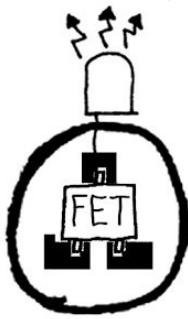
4. solder LED (-) leg to the transistor drain (D).
